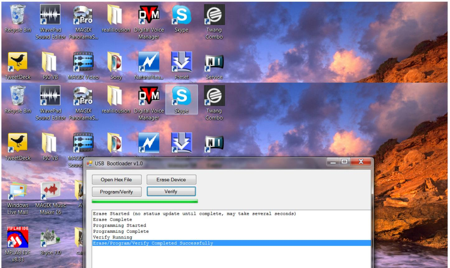
The Boot loader screen will show the steps taking place and tell you the program was uploaded successfully on the last line of the boot loaders display. Disconnect your Ovilus X from your USB port. Your Firm ware Upgrade will be ready to use.
