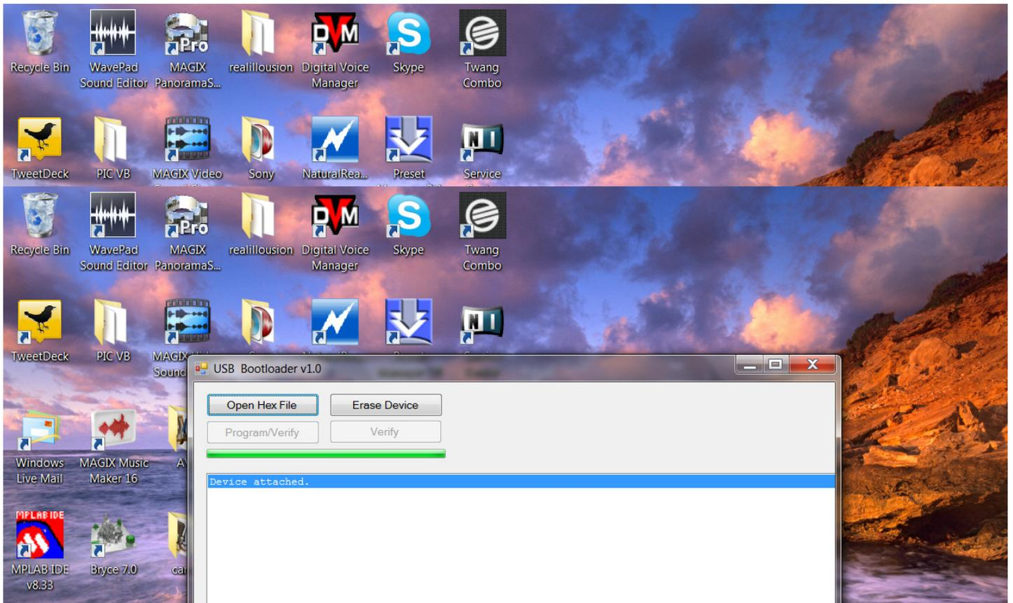
Power off the Ovilus X, Connect the USB cable to your computer. While pressing the Mode Button on the Ovilus X Connect the the USB cable to the Ovilus X. The Two Led's on the right side of the Ovilus X will begin to flash , release the mode switch.
