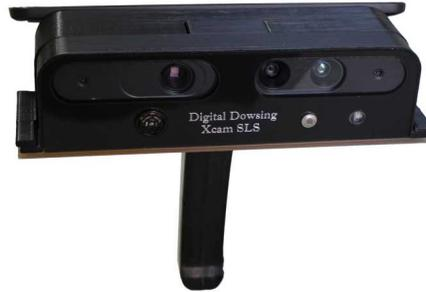
All of the data is gathered and displayed in real time. The connected PC based tablet gathers all the data into one central program for simple viewing and recording. One single screen shows all your data: Temperature, Imaging, Audio Range, Distance, Light Levels and Visualized Object Scanning.
